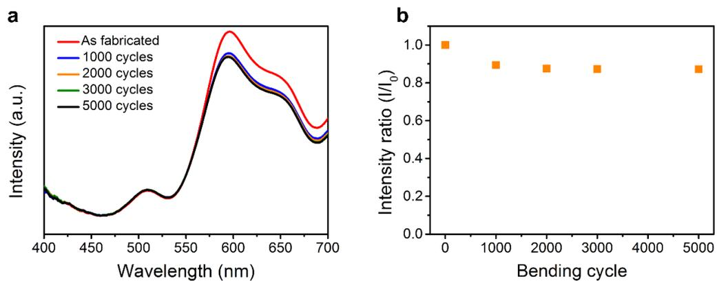
**Figure S3. a)** Spectrum of the orange fiber electrode over 5000 bending cycles with a bending angle of 180°. **b)** Correlated spectrum variation of intensity peak value in **a**.
