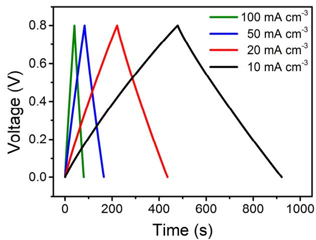
**Figure S6.** Galvanostatic charge-discharge curve of a fluorescent supercapacitor fiber based on MWCNT/PEDOT composite at increasing current densities from 10 to 100 mA cm<sup>-3</sup>.
