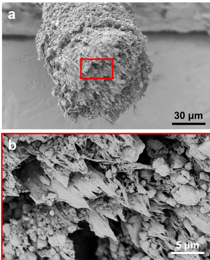
**Figure S2.** a) Cross-sectional SEM image of the fluorescent fiber. b) Higher magnification of the region marked with a red rectangle in a.
