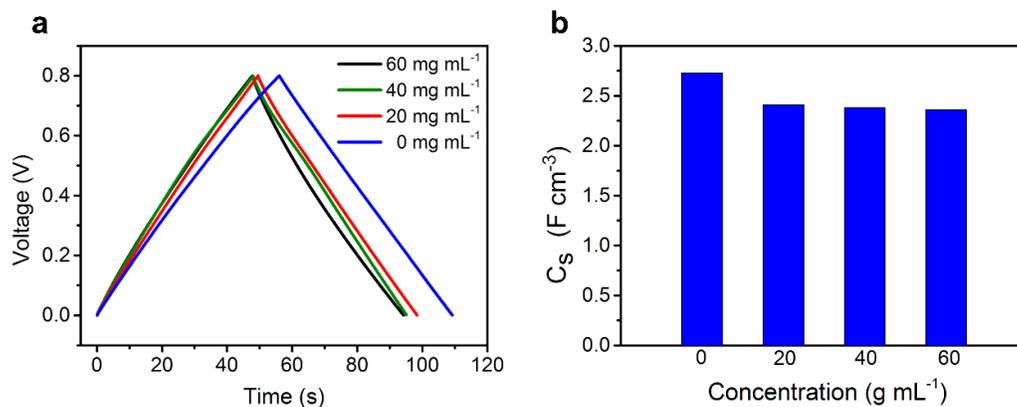
**Figure S5.** a) Galvanostatic charge-discharge curves of fluorescent supercapacitor fibers incorporated with increasing dye dispersion concentration from 0 to 60 mg mL<sup>-1</sup>. Current density, 10 mA cm<sup>-3</sup>. b) Dependence of specific capacitance on the incorporated dye dispersion concentration.
