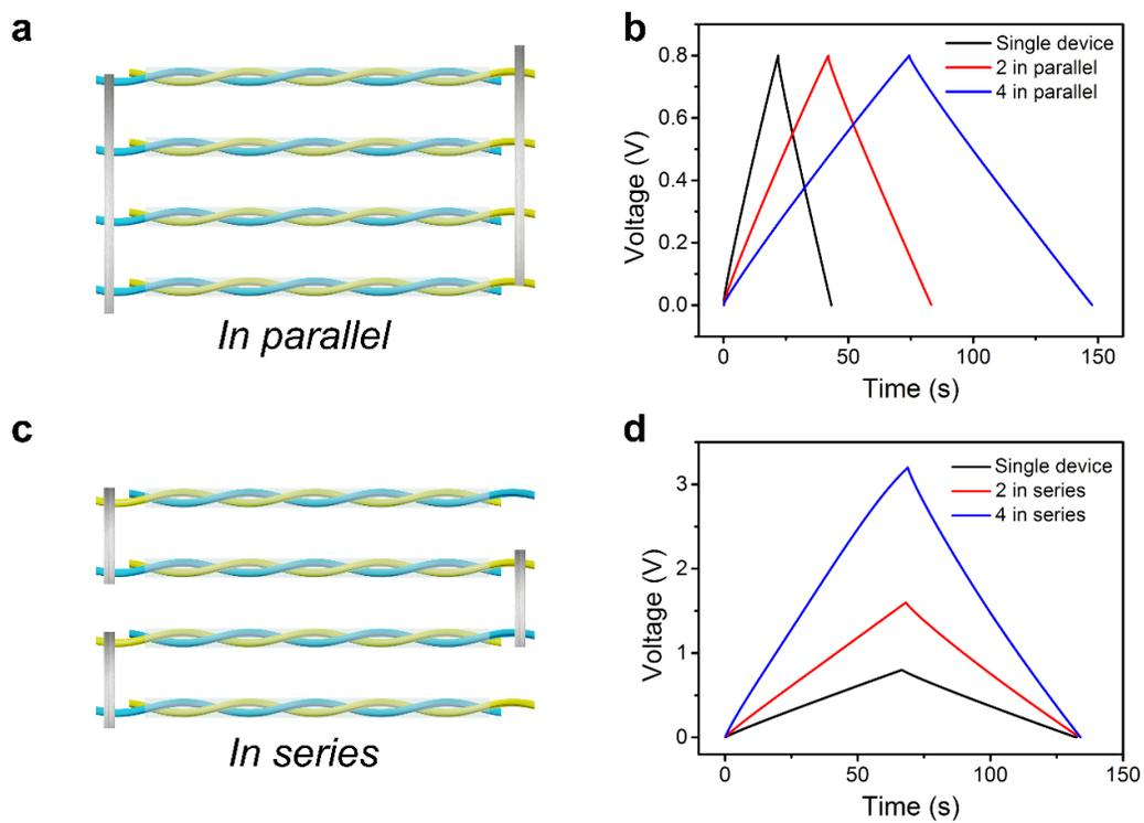
**Figure S8.** Schematic illustrations of the integrated configurations and corresponding galvanostatic charge-discharge curves of the fluorescent supercapacitor fibers. **a, b)** Increased power capacities by connection in parallel. **c, d)** Increased voltage by connection in series.
