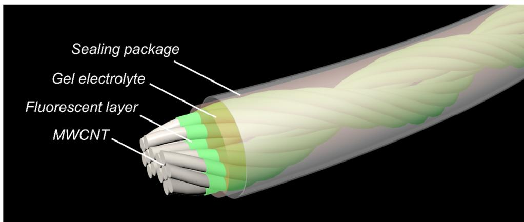
**Figure S1.** Schematic illustration to the components of the fluorescent supercapacitor fiber.
