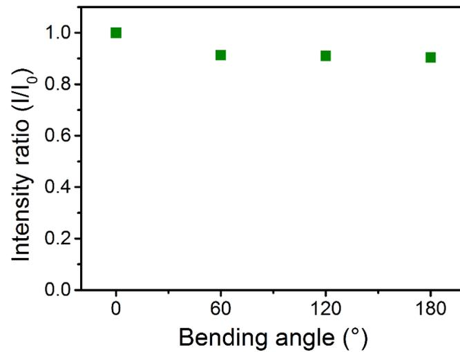
**Figure S9.** Spectrum peak value variation of an unpackaged green fluorescent supercapacitor fiber under bending with increasing bending angles from 0 to 180°.
