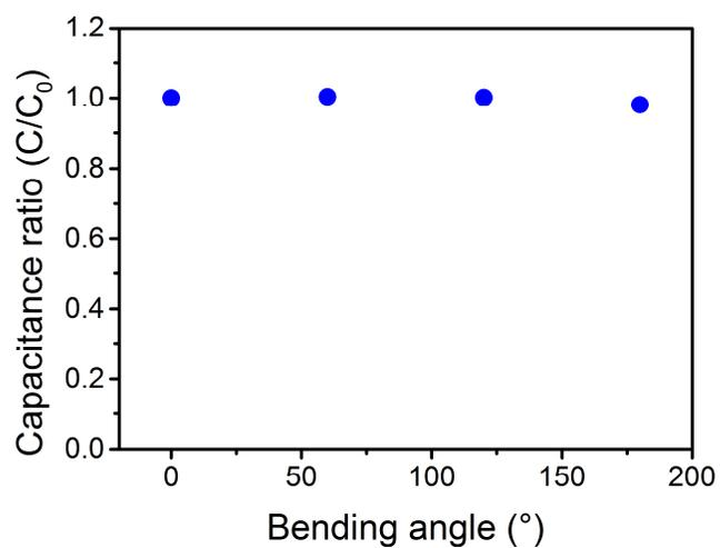
**Figure S10.** Capacitance variation of a fluorescent supercapacitor fiber under bending with increasing bending angle from 0 to 180°. Current density, 10 mA cm<sup>-3</sup>.
